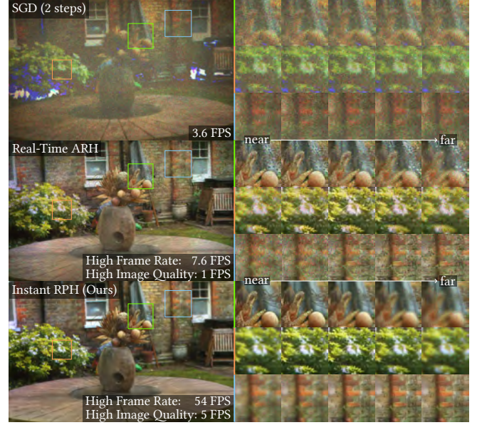
Fig. 2. Real-Time Random Phase Holography. Existing random phase holography methods are bounded by a strict trade-off between speed and image quality. To achieve interactive rates, iterative solvers significantly sacrifice quality, yielding very poor results (top). The recent ARH [Chu et al. 2025] struggles in both image quality and runtime when scaling up focal resolution (middle). Our Instant RPH overcomes this trade-off, synthesizing high-quality 3D holograms with natural defocus and parallax (bottom).
