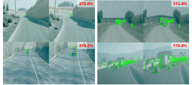
Figure 5. Learned hyperbolic foveated transform on the Truck-Drive dataset. The original image (left) and the foveated image (right) are shown, together with the percentage increase in object bounding-box area. Both views are cropped to the same image region, highlighting the local magnification induced by the foveation transform. The proposed transform is effective for both isolated targets and dense, busy scenes.
